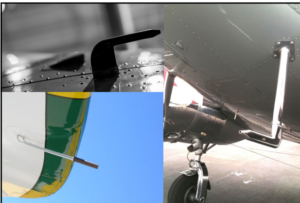
Pitot tube – Lost_in_the_Midwest (Adobe Stock) Pitot tubes – Brave Heart (CC BY-NC-ND 2.0) Pitot tube (Lockheed 12A Electra, 1939) – Brave Heart (CC BY-NC-ND 2.0)
